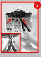
Use needle nose pliers to unhook the 2 sets of plastic clips at the back of the black tray.
